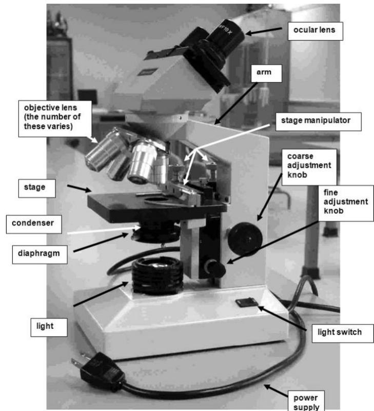
A magnifying glass is a simple microscope because it consists of only one lens. This microscope is called compound because it consists of two or more lenses. The two lenses on the microscope are called the ocular lens (the eyepiece, or lens closest to your eye) and the objective lens (the lens that is variable and can be changed). The ocular lens typically magnifies objects 10 times, whereas the objective lenses (used one at a time and mounted on a nosepiece) vary from 4 to 100 times.
